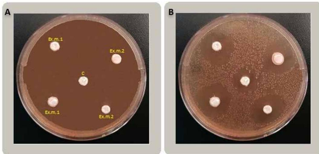
**Figure 4: A. Placement of discs before incubation. Left: Two discs experimental materials I (Ex. M.1). Right: Two discs experimental material II (Ex. M.2). Middle: One disc control (C). B. Discs of the tested materials surrounded by the inhibition zone.**
