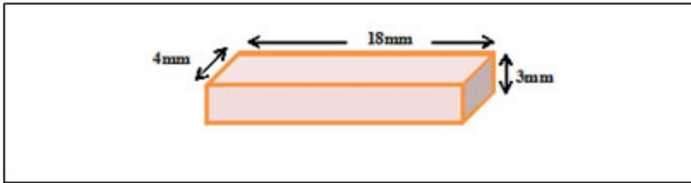
Figure 1: The prepared all-ceramic sample dimensions.
