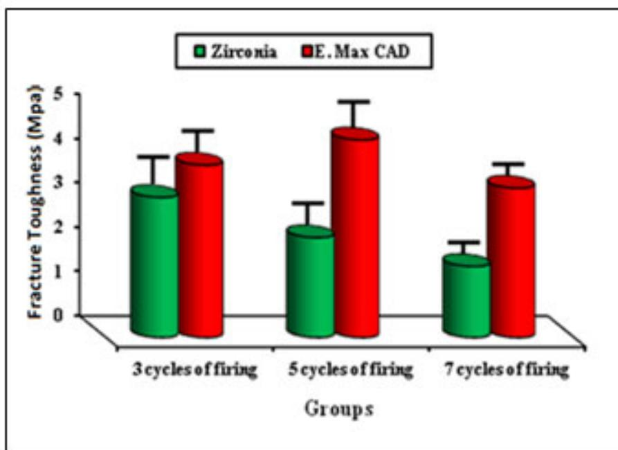
Figure 3: Mean values for Fracture Toughness test distributed in different groups.
