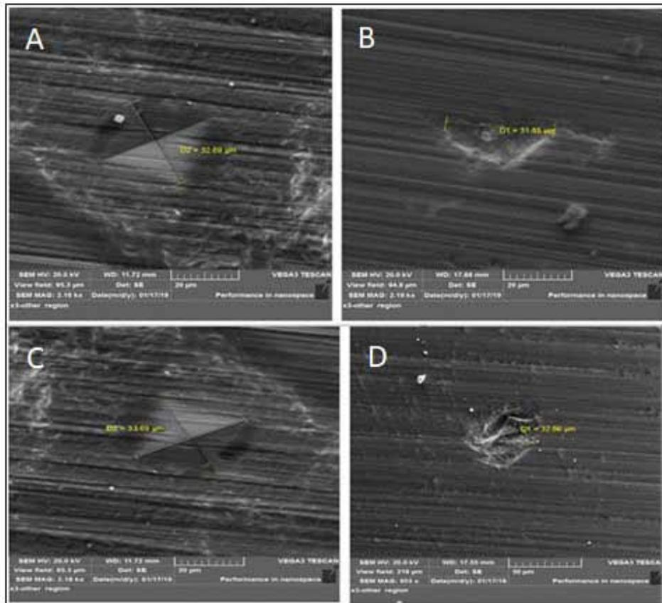
**Figure 4: SEM image for both materials: A- Zirconia without firing. B- Zirconia with 3 cycles of firing C- IPS e. max CAD without firing. D- IPS e. max CAD with 3 cycles of firing.**
