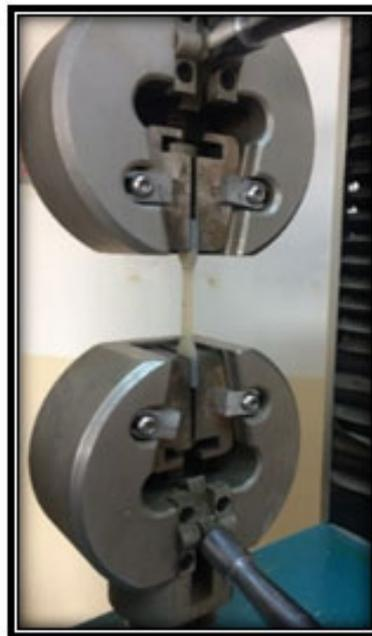
Figure 3: Specimen under tensile test.
