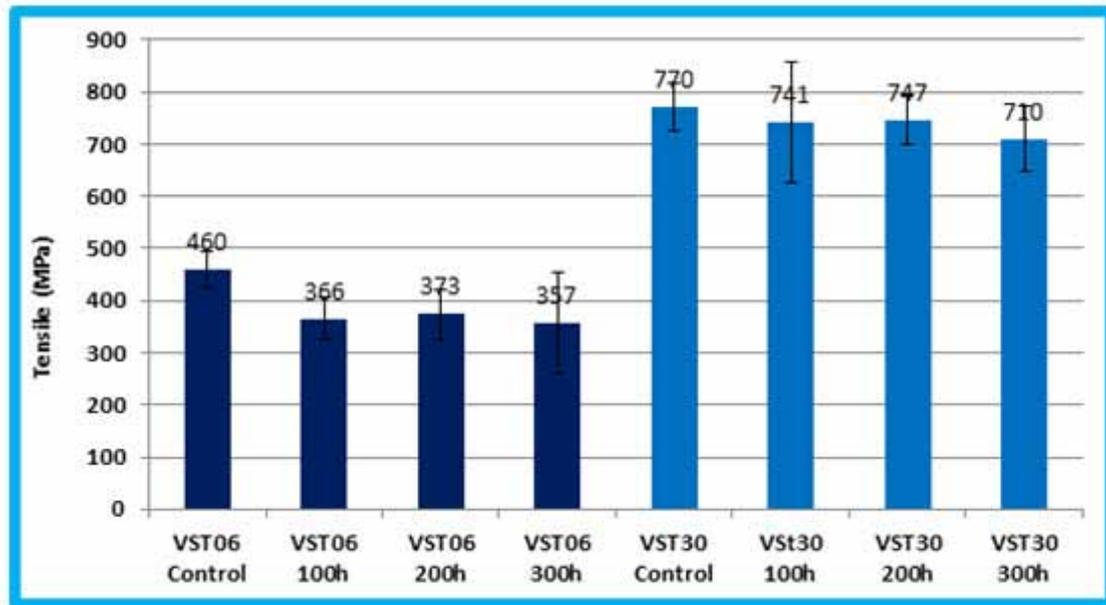
Figure 4: Mean values and standard deviation of tensile strength test for all study clear groups of VST-30 and VST-06.
