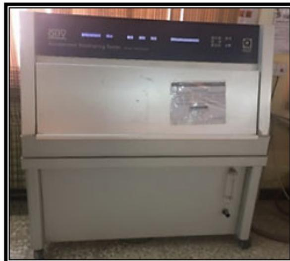
Figure 2: Weather-Ometer device (QUV).
