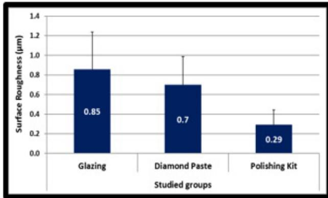
**Figure (2): Bar chart showing the mean distribution of surface roughness (Ra) in  $\mu\text{m}$  for the studied groups.**
