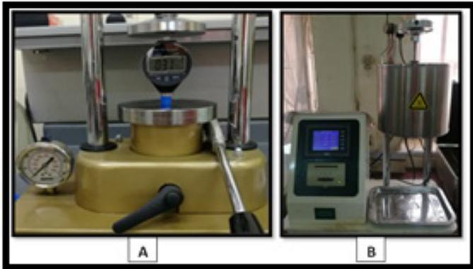
Figure (2): A: Surface hardness device (Shore D); and B: Melt flow index tester device.
