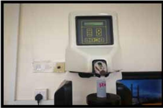
**Figure (5): Rockwell hardness tester.**
