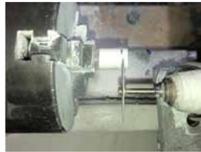
**Figure (1): Milling of zirconia specimens.**
