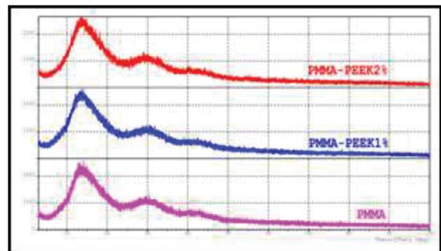
**Figure 4: Diagram shows the XRD pattern of PMMA base resin, PMMA/1%PEEK, and PMMA/2%PEEK prepared study material.**
