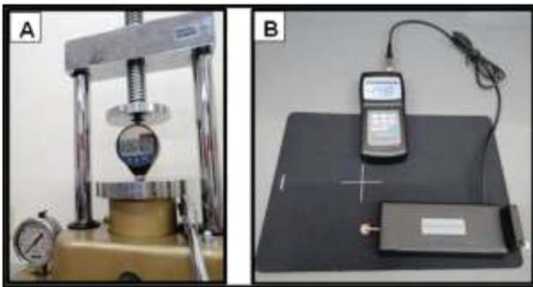
**Figure 1: A, Shore D durometer surface hardness unit; and B, Surface roughness profilometer tester device.**
