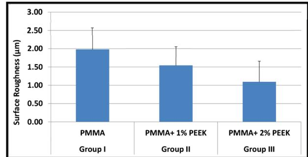
**Figure 3: Mean distribution of the surface roughness of the tested groups.**
