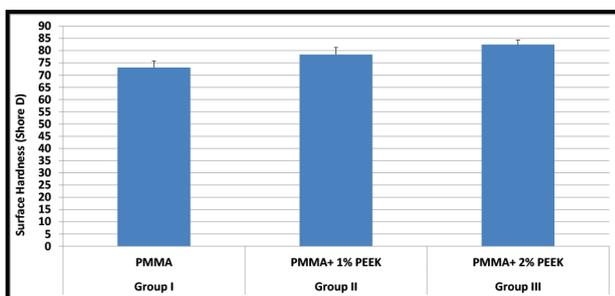
**Figure 2: Mean distribution of the surface hardness of the tested groups.**
